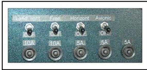
Example of switch and fuse layout
