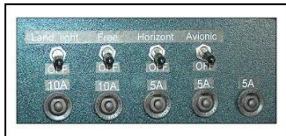
Example of switch and fuse layout
